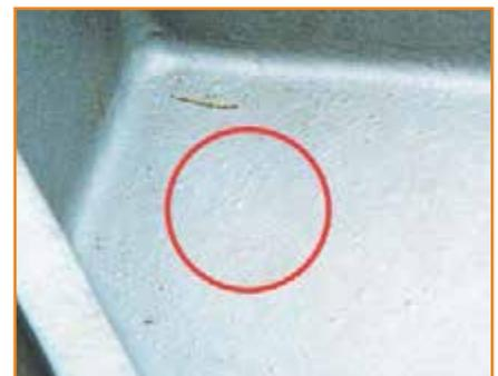
Blasters cleaning up abrasive can easily miss some – see the lumps under the coating?
