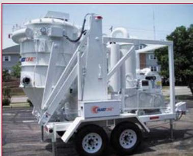
A trailer mounted Vacuload™ with self lifting vacuum unit – no cranes required.
