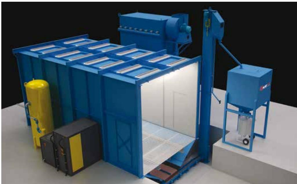
Bucket elevators have the disadvantage of costing a little more initially, but a bucket elevator cannot bog down once the flow control gate is set. You will need to replace the buckets every few years depending on usage.
