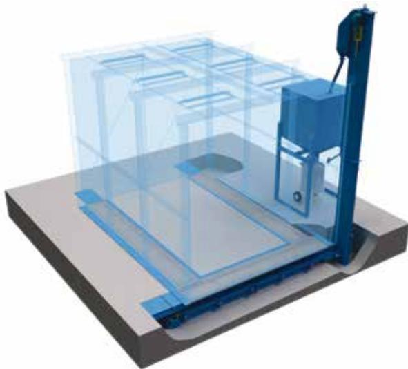
**Sweeper Floors, Augers, Conveyor Belts** have been grouped together in this publication as they are a form of conveying which is being used less frequently. Although they use considerably less power than the pneumatic recovery systems, they have not achieved a reasonable standard of reliability, with broken cables, sweepers and augers when jams occur. High wear due to the scraping action and dust
