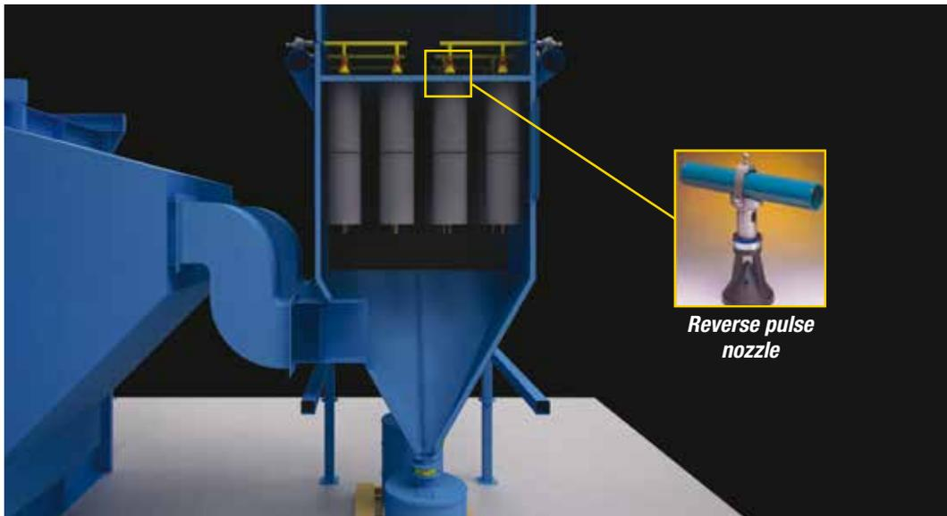
A sequential timer activates an air solenoid valve which sends a “shock” of compressed air through the element or bag in the opposite direction to air flow. If the shock is sufficient, dust which has accumulated on the outside will be released and most should fall away, even while the dust collector is operating. It is an especially good idea to continue the pulse for several cycles after the dust collector fan is turned off.
