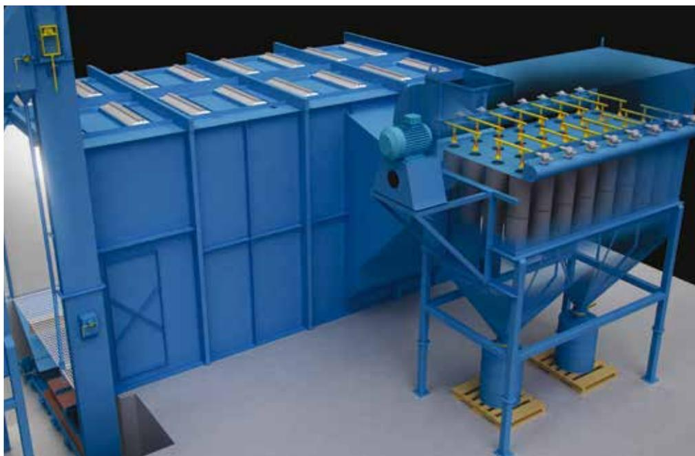
Mechanical shakers have been employed to shake and loosen dust from filter bags when the dust collector is turned off. This is necessary as the fine dust clogs the bag, reducing airflow dramatically.
