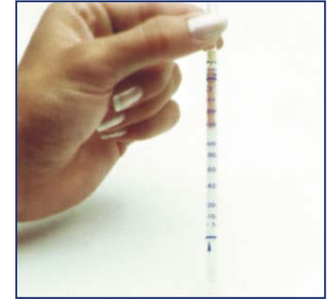
Step 6 Wait approx 1 1/2 minutes or until the solution has wicked-up to the top of the titrator tube. The cotton at the top of the tube will change colour (amber) when fully saturated.
