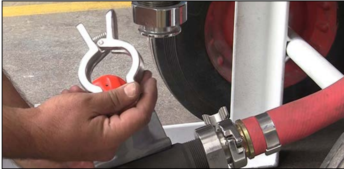
Removing a Triclover to separate the metering valve and the blast pot.
